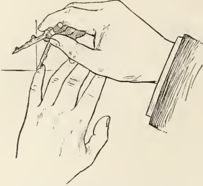
FIG. 26.—Setting the compass.
